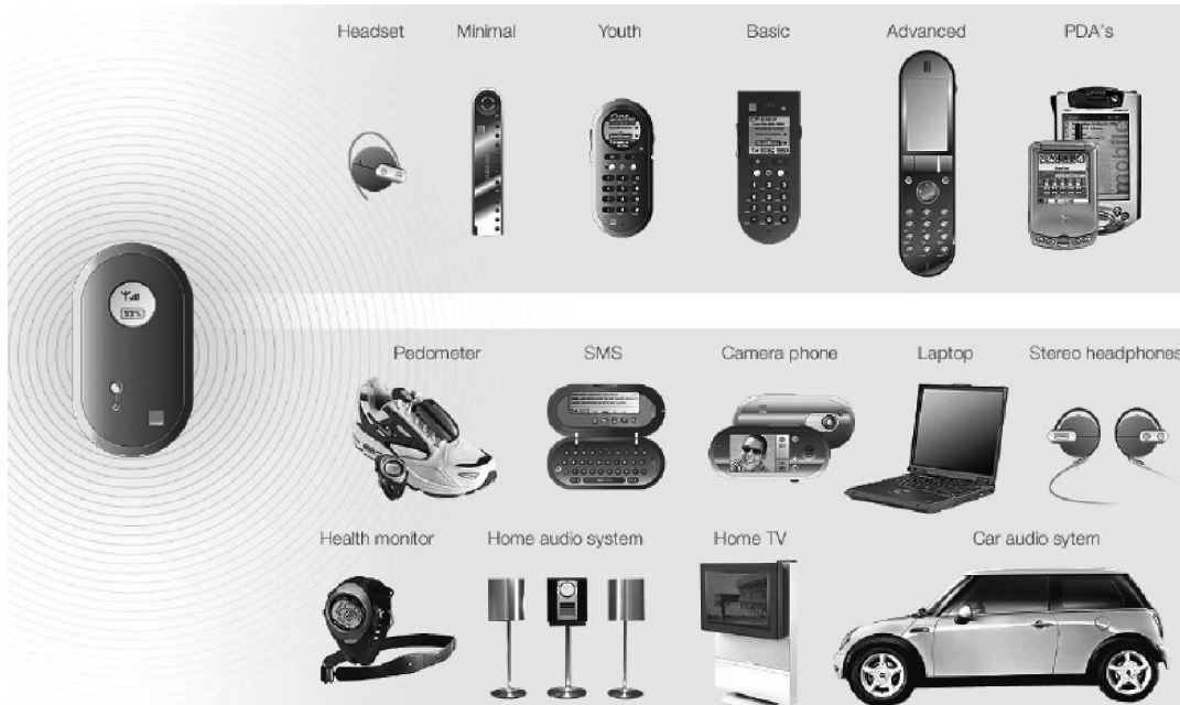
Figure 7. The Cellular Hub is essentially a wireless phone with data capability, to which various devices connect by using the Bluetooth wireless protocol.
