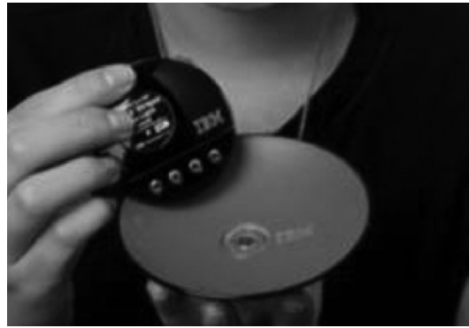
Figure 2 and 3. Inspired by the culture of China, this prototype MP3 player uses the metaphor of a meditation stone for the device and a rice bowl for the charger/download base. These are familiar metaphors to customers in China, but refreshing and new for global markets.
