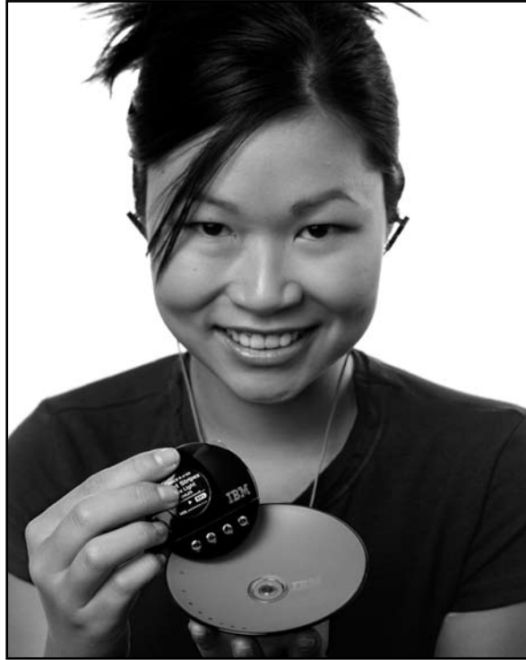
Inspired by the culture of China, this prototype MP3 player uses the metaphor of a meditation stone for the device and a rice bowl for the charger/download base.
